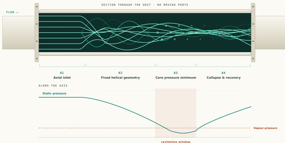
FIGURE 1 · Section along the flow axis. Fixed internal geometry converts axial momentum to tangential momentum; the resulting radial pressure gradient drops static pressure at the vortex core below local vapor pressure, nucleating cavities that collapse as pressure recovers downstream of the throat. Downstream, treated water exhibits lower surface tension, which reads in soil as faster infiltration and a wider, deeper wetting front.
